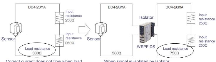
Correct current does not flow when load resistance of sensor output is not enough.
