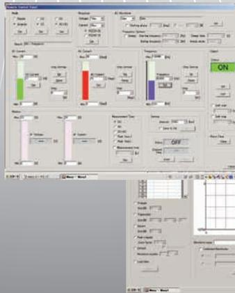
"Remote Control Panel" works as graphical remote controller for power supplies and electronic loads, with Monitoring and data logging function.
