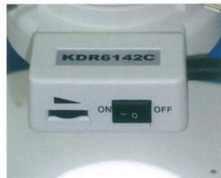
Lighting module and adjustment parts integrated 光量調節跟照明模組一體化
