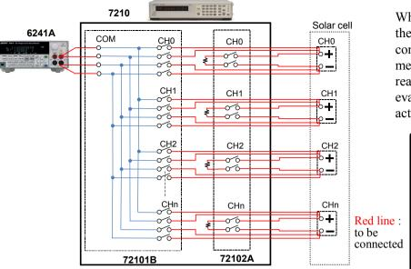
When load resistances are connected to the scanner by using the actuator card, connecting channels other than ones to be measured to the load resistances will realize degradation characteristic evaluation under a condition close to the actual use condition.
