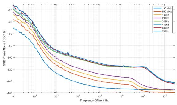
Measured SSB phase noise for different carrier frequencies, with R&S®SMCVB-K709 option
