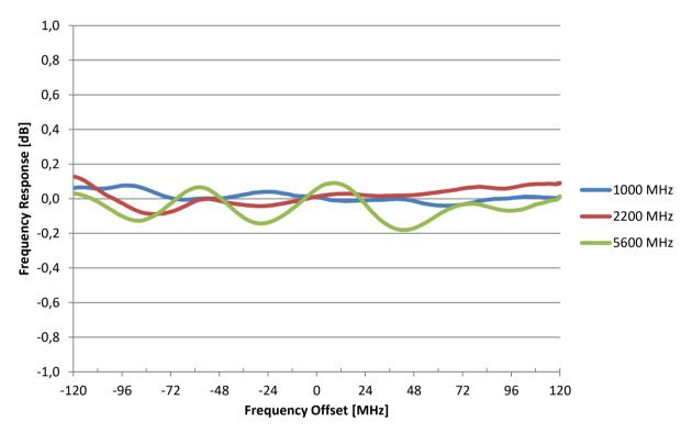
Measured RF modulation frequency response at different carrier frequencies
