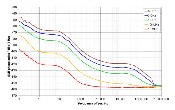
SSB phase noise with the R&S®SGT-B1 internal OCXO option (meas.)
