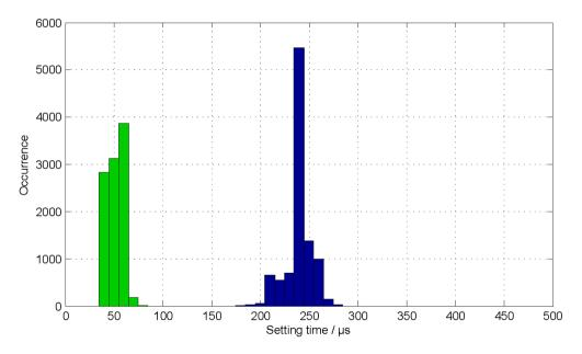
Histogram of level setting times measured via PCIe/Ethernet interface, I/Q modulation from internal baseband, setting characteristic: auto. Green: with digital attenuation. Blue: with arbitrary level setting.
