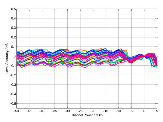
Level linearity for internally generated LTE uplink signal at various test frequencies (meas.)
