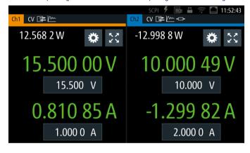
The R&S®NGM200 power supplies have a circuit design that allows the user to determine how the power supply regulates load changes. The "Fast" default setting is optimized for speed, achieving recovery times of  $< 30~\mu s$ . Deactivating "Fast" slightly increases the recovery time, focusing on preventing overshoots under special load conditions.
