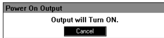
Figure 4-24 The Message Window to be Shown Before the Automatic Output-On After the Power-On
