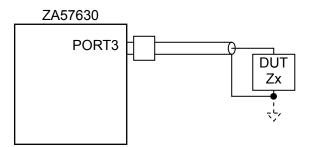
Figure 4-6 Impedance Measurement Connection Example 5 (IMPD-2T)
