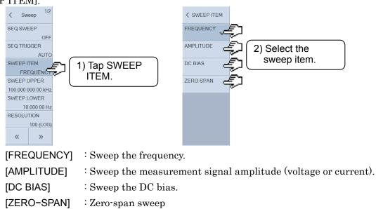
In the case of the measurement signal amplitude sweep, whether voltage amplitude or current amplitude sweeping is performed is determined by whether the setting unit of the measurement signal is voltage or current. Refer to "**■** Setting the amplitude and DC bias unit" in "4.3 Setting Measurement Signals".
