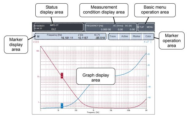
Figure 3-13 Screen Immediately after Startup
