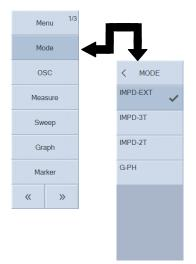
This menu sets the measurement mode of this instrument.
