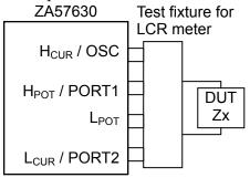
Figure 4-4 Impedance Measurement Connection Example 4 (IMPD-3T)
