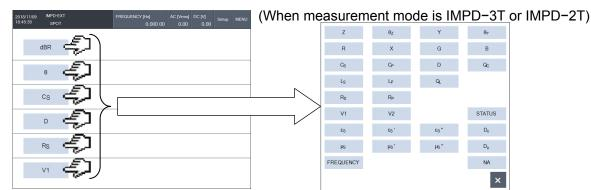
If you select [NA], that parameter will be hidden (only PRMTR3 to 6). The types and formulas of parameters other than [STATUS] are the same as for sweep measurement. Refer to Table 4-3 and Table 4-6.
