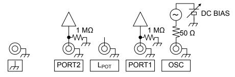
Figure 3-3 Functions of Measurement Connectors (Measurement Modes IMPD-EXT and G-PH)
