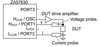
$\circ$  Connection example for measurement mode IMPD–3T
