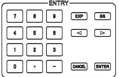
This is a set of keys for entering the numeric values of setting parameters.
