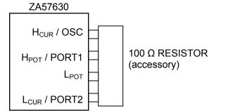
Figure 4-5 How to Check Operation Using 100  $\Omega$  RESISTOR (IMPD-3T)
