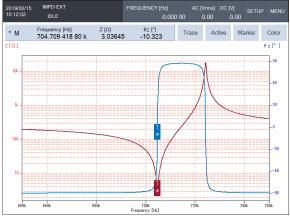
8) Operating the knob moves a marker on the measurement data. This allows you to read the measurement value at any frequency. You can also perform operations such as detecting the maximum value, searching, and finding the location of an arbitrary gain value. For more details on the operations, refer to "1.7 Marker Operations" in Instruction Manual (Advanced).
