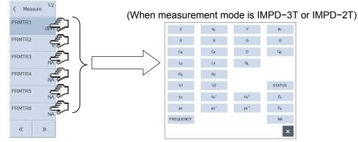
Tap the menu to display a palette listing the parameters that can be measured. Tap to select the parameters to measure and display in the palette. The measurement and display items can also be changed by tapping the parameter buttons in the spot measurement result screen.
