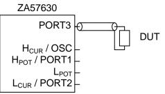
$\circ$  Connection example for measurement mode G–PH
