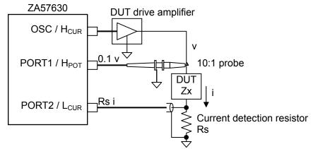
Figure 4-1 Impedance Measurement Connection Example 1 (IMPD-EXT, Measurement of High Voltage)
