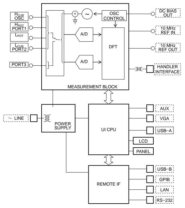
Figure 1-1 Block Diagram
