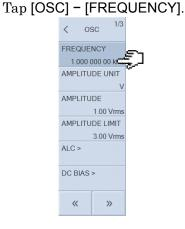
Tap a function key at the bottom of the LCD to set the frequency setting.
