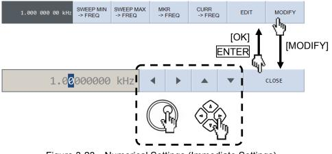
Figure 3-23 Numerical Settings (Immediate Settings)
