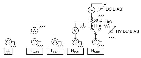
Figure 3-4 Functions of Measurement Connectors (Measurement Mode: IMPD-3T)
