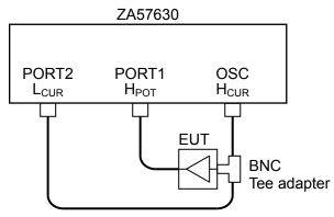
Figure 4-7 Gain and Phase Measurement Connection Example
