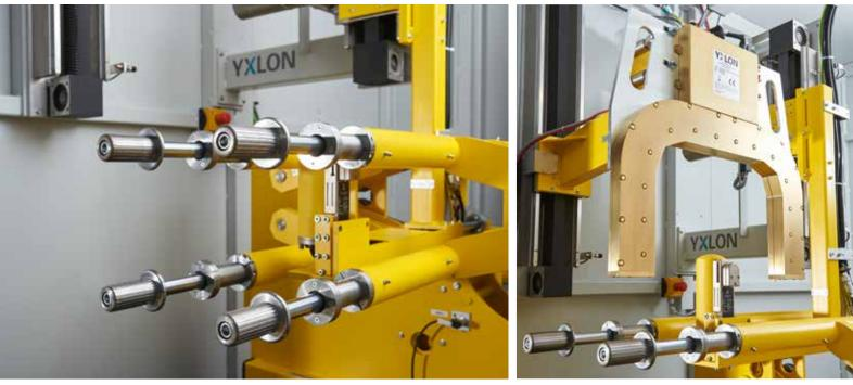
The four-spindle manipulation ensures for reliable and repeatable inspection results.
