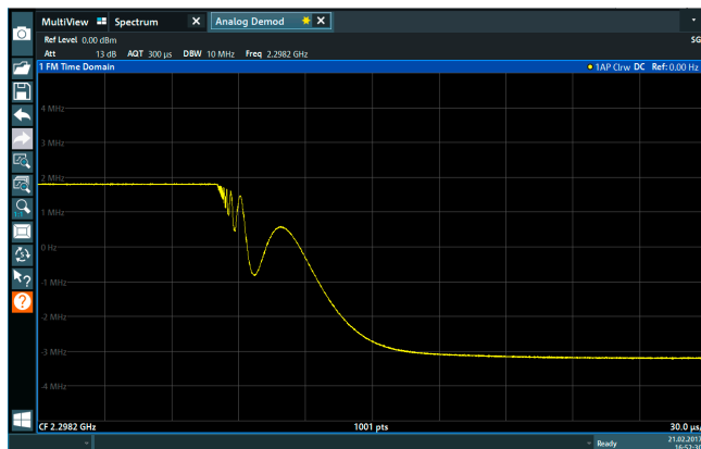
Frequency settling behavior of an oscillator
