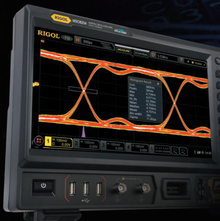
Perform eye measurement on the 622 Mb/s signal.
