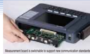
Measurement board is switchable to support new communication standards.
