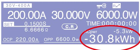
The current regenerated power value is shown in the upper row of the section, while the accumulated regenerated power value is presented in a larger font in the lower row. (The minus (-) sign indicates power regenerated.)
