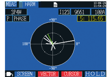
Harmonic power phase angle graph screen
