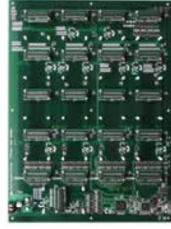
Example of a custom burn-in board
