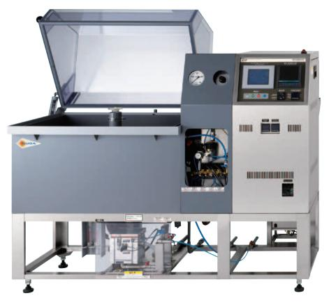
CYP-90 is an accelerated corrosion test apparatus for metallic materials and coatings, capable of salt spray, dry, wet, or ventilation tests either singularly or in cycles. CYP-90 is used in various industries around the world as the standard model to be able to conduct cyclic tests specified in JIS, JASO, and ISO. It can simulate accelerated degradation in excellent correlation with outdoor exposure. CYP-90 is the most
