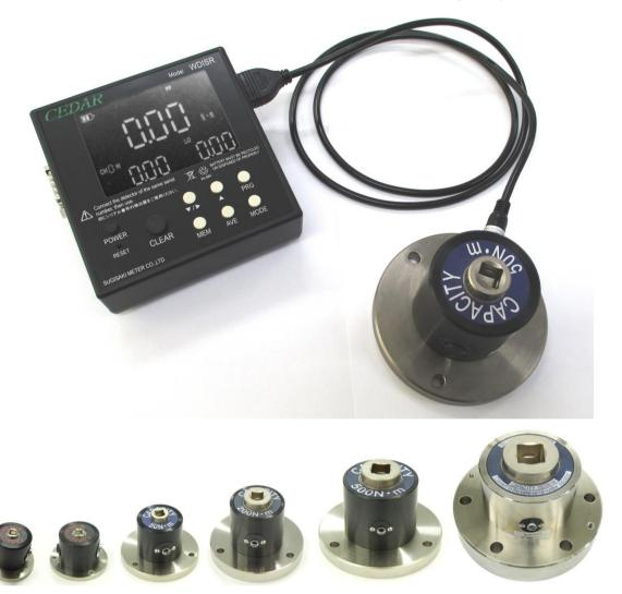
It works with a personal computer or PLC to manage torque measurement more highly. For managing manual torque drivers and wrenches.
