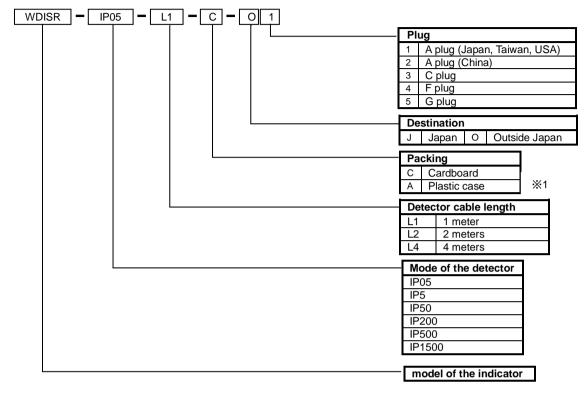
1 If you select the detection unit IP200, IP500, or IP1500, the attache case (-A) cannot be used.
