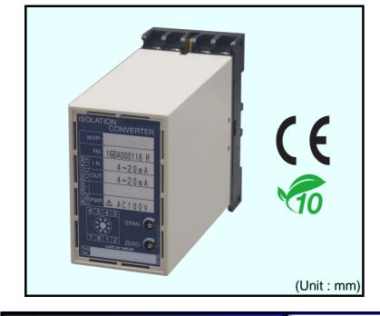
This plug-in type converter (isolator) provides signal output which is mutually isolated between input, output and power-supply. It amplifies and converts various kinds of signal with isolation to use in the integrated instrumental control system. It is highly effective as noise countermeasures.
