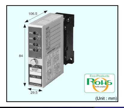
This compact plug-in converter receives a pulse train signal and converts into analog signal that is proportional to its frequency, and provides two isolated outputs.
