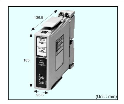
This slim-type plug-in converter accepts a RTD input and provides optically isolated DC voltage or current outputs.
