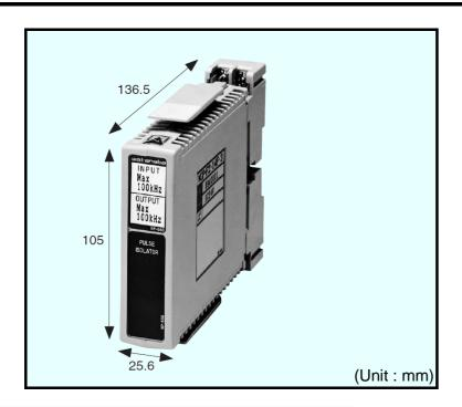
This slim-type plug-in converter (pulse isolator) receives a pulse train signal extracted from the sensor or control equipment, adds waveform shaping, insulation, and level conversion, and then outputs two pulse string signals.
