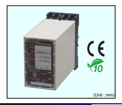
This plug-in, high-speed response type converter (isolator) provides signal output which is mutually isolated between input, output and power-supply. It amplifies and converts various kinds of signal with isolation to use in the integrated instrumental control system. It is highly effective as noise countermeasures.
