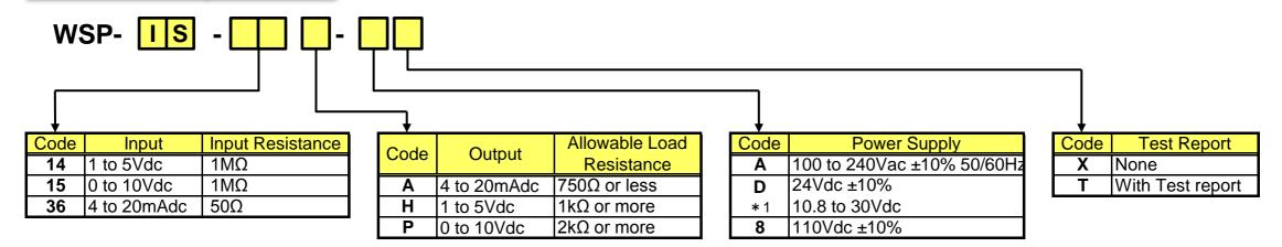
\*1···CE approval do not adapt when power supply is 10.8Vdc to 30Vdc.
