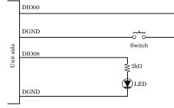
When switch is "ON", the corresponding bit is "0". When switch is "OFF" in contrast, the corresponding bit is "1". When "1" is output to a relevant bit, the corresponding LED comes on. When "0" is output to the bit, in contrast, the LED goes out.
