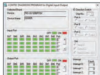
A sample screen of checking digital input/output
