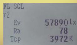
Illuminance Ev / Average color rendering property evaluation Ra / Correlated color temperature Tcp mode
