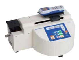
The MODEL-2252RDH is designed to measure the adhesion strength of electronic parts mounted on horizontal boards. The sample fixing position may be adjusted in the Z direction. The digital force gage RZ-20 is mounted on the force measuring side and the shearing jig is mounted at the top. It is also possible to mount the hot plate (HTP-OP-1)on the sample fixing side. The force measuring unit of this tester moves to the right and left. It stores measured data, which may be printed or read in a PC.
