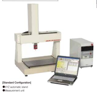
This tester is dedicated to feeling tests of force-displacement of various switches, keyboard switches, dome switches, rubber switches, etc. Three axes of X, Y and Z can be controlled automatically. The tester is capable of testing 16 ON/OFF contacts maximum. The tester is equipped with a jog dial to facilitate teaching. Waveforms are displayed in real time on the amplifier and PC screen.
