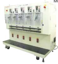
This is designed for durability tests of cables in conformity to the UL and JIS standards. It stops operation automatically at the set values (±90° & ±45°) and when the cable is broken. (Interlock type and manual type are available.)
