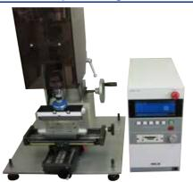
This tester is designed to test a correlation between torque value and the rotation angle. The acquired torque value and angle data are drawn on a torque-angle graph. It is also possible to automatically acquire the click torque value and angle during turning and show typical measurement values (click values).
