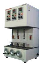
The MODEL-SR-3 is designed for durability tests of various electronic parts. It automatically stops a test at the preset cycle or when a test work is broken.
