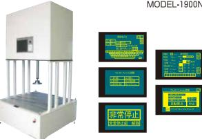
The MODEL-1900N allows all test patterns to be set on the touch panel. It stores a maximum of ten JIS, JAS and any optional patterns in the memory unit, which may be read out in tests. The test data are displayed on the screen and may be printed out.
