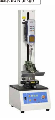
The MODEL-1308U/NF is a low-price and compact JIS-rated lead-free solder tester. It is designed for 45° pull tests of QFP lead solder and shearing tests of chip parts, which are enabled by replacing the jigs and RZ series digital force gages. Measured data are stored in the RZ series digital force gage and may be printed out or loaded into a PC after completion of measurement. The jigs are commonly used for the MODEL-1605 VC/NF.
