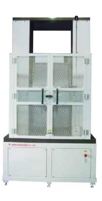
The MODEL-1431VC Series are multi-purpose large-size force testers designed for compression, tensile, bending and other tests of various large works at 1, 2, 5, 10 and 20 tonf. They employ precision ball screws and servo motors in the driving mechanisms and rotary encoders for displacement detection.
