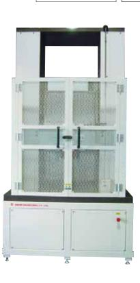
The MODEL-1431VC Series are multi-purpose large-size force testers designed for compression, tensile, bending and other tests of various large works at 1, 2, 5, 10 and 20 tonf. They employ precision ball screws and servo motors in the driving mechanisms and rotary encoders for displacement detection.
