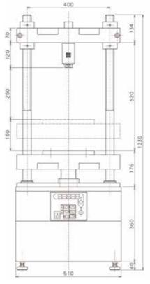
These models are large size testers designed for compression and tensile force tests up to 500 to 2000Kgf (5 to 20kN). They use the MODEL-1016C amplifier and display the measurement results on LCD panels.
