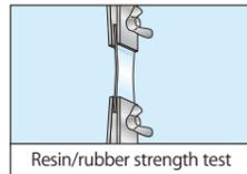
Resin/rubber strength test
