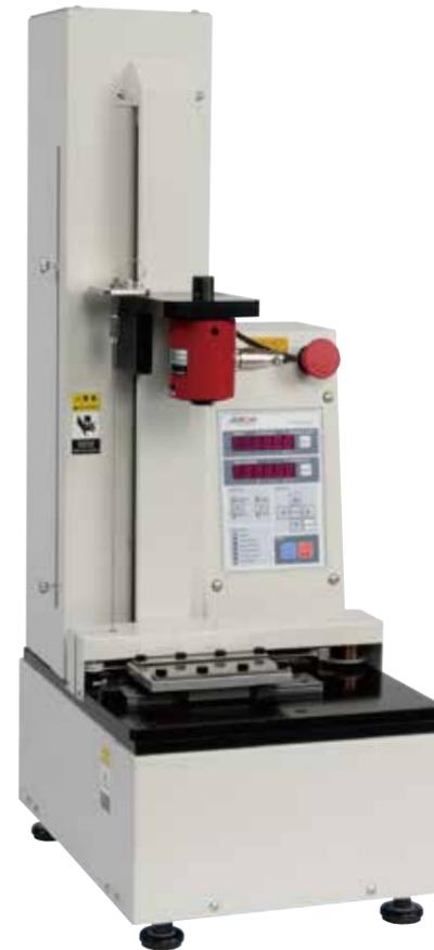
This is a low priced adhesion tester based on FTN1 - 13A with only the mechanism changed. The maximum test speed has been increased to 1000 mm/min to meet needs of high-speed tests. In addition, a jig for 90-degree peeling that meets testing in accordance with JIS Z 0237 and software FTN-2008P dedicated to adhesion test are also available.
