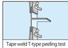
Tape weld T-type peeling test
