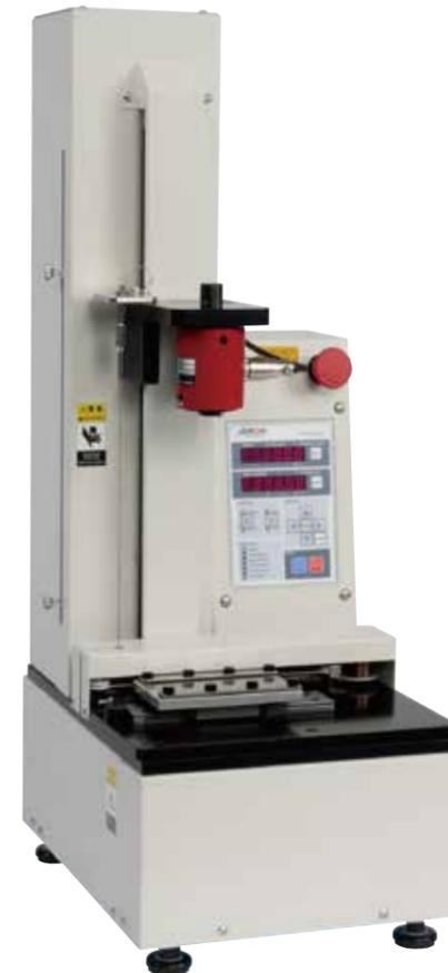
This is a low priced adhesion tester based on FTN1 - 13A with only the mechanism changed. The maximum test speed has been increased to 1000 mm/min to meet needs of high-speed tests. In addition, a jig for 90-degree peeling that meets testing in accordance with JIS Z 0237 and software FTN-2008P dedicated to adhesion test are also available.
