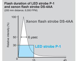
Xenon lamp strobes feature instantaneous flash light of high intensity. LED strobes emit a large amount of light by adjusting the flash duration.
