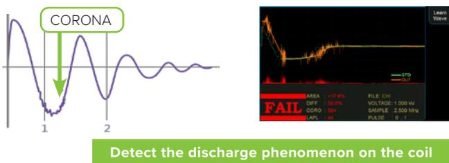
Detect the discharge phenomenon on the coil
