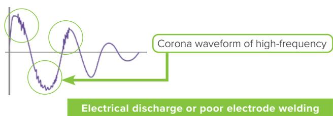
Electrical discharge or poor electrode welding
