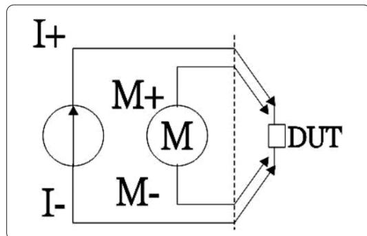
4-wire measurement, avoiding the resistance issues caused from adapting the fixture wires, low resistance of 1mΩ.
