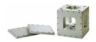
The JSA series cubic style fixture is used for performing vibration test of relatively small and light specimen such as various sensors, electrical components including electronic parts, printed circuit boards. In addition, we design and produce fixtures that meets the requirements for strength, stiffness, resonance frequency by taking the mass of a test article and frequency range of the vibration testing system into consideration.
