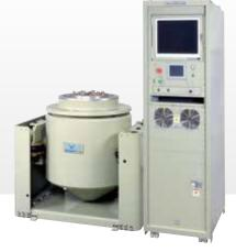
The FV series system responds to shock test conditions; Shock Pulse Duration 11 ms & Level 980 m/s² (100 G)
