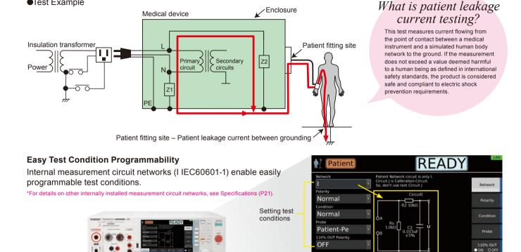
Measurement circuit network (network I IEC60601-1)
