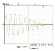
The fall time control feature allows you to gradually decrease the test voltage after a successful AC/DC hipot test. The voltage fall time can be set from 0s to 200s at a resolution of 0.1s. (OFF is also selectable).
