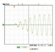
The rise time control feature allows you to gradually increase voltage to a set value while AC/ DC hipot tests are conducted. Voltage rise times can be set from 0.1s to 200.0s at a resolution of 0.1s.
