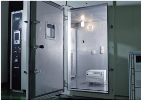
Temperature & Humidity Cycle Test Chamber
