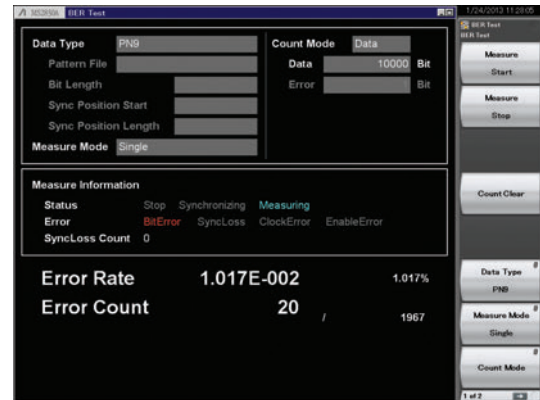
BER Measurement Function Main Screen
