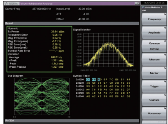
4FSK Modulation Analysis Measurement Example
