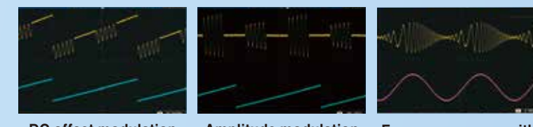
DC offset modulation (Rising ramp waveform) Amplitude modulation (Rising ramp waveform) Frequency sweep with amplitude modulation
