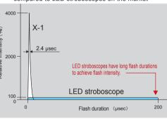
(Tested at flash frequency 3000 FPM and at a 300 mm distance.)
