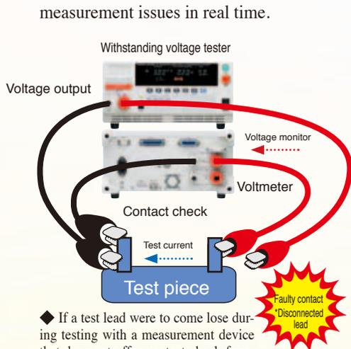
◆ If a test lead were to come loose during testing with a measurement device that does not offer contact check functionality, defective test pieces would be judged to be non-defective.
