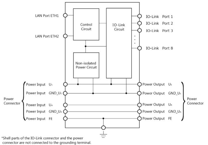
\*Shell parts of the IO-Link connector and the power connector are not connected to the grounding terminal.
