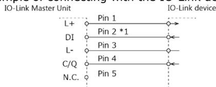
\*1 As for an IO-Link device without a Pin 2 digital input function, it will be unconnected on the IO-Link device side and digital input data will be always off.
