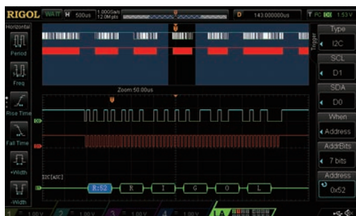
Deep memory depth for the digital channels, serial bus trigger and decoding on digital channels
