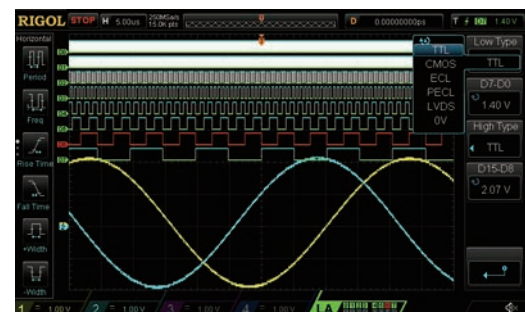
Supports a variety of logic levels
